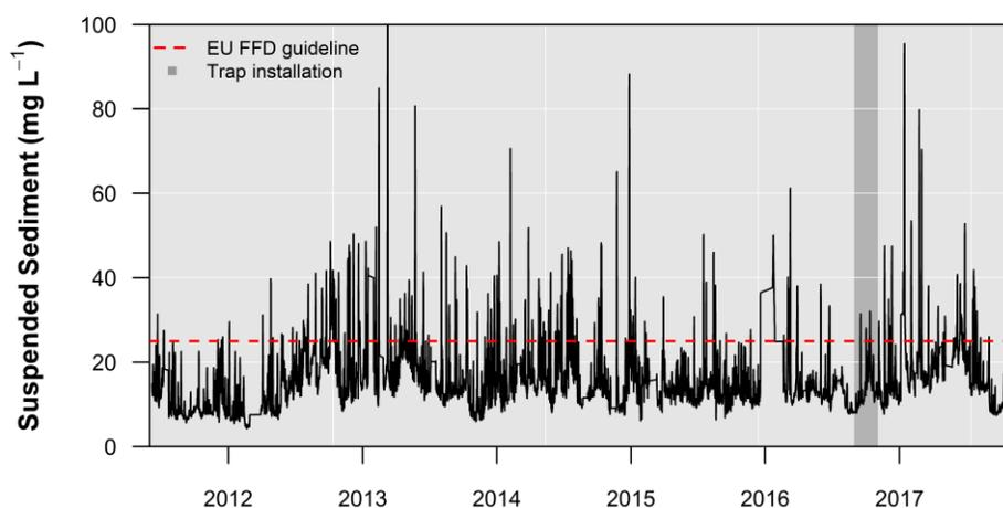
**Figure 1:** Suspended sediment concentrations recorded in the River Blackwater downstream of the roadside sediment traps before (June 2011 – August 2016) and after (November 2016 – October 2017) trap installation. The European Union Freshwater Fisheries Directive (2006/44/EC) guideline maximum value of  $25 \text{ mg L}^{-1}$  in waters suitable for salmonid and cyprinid fish populations is also shown.
