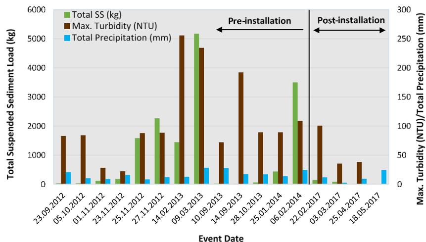
**Figure 2: Total suspended sediment load and maximum turbidity values recorded in the River Blackwater downstream of the sediment traps during 18 precipitation events (13 prior to trap installation, 5 post installation) between 2012 and 2017.**
