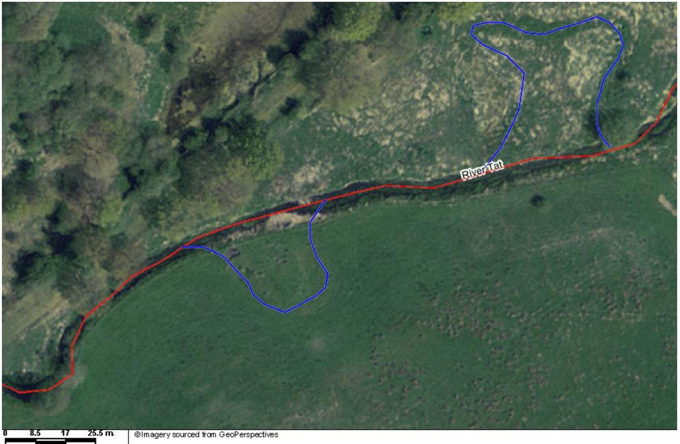
Meander restoration on the River Tat. The red line shows the pre-restoration course of the river. The blue lines show the location of former meanders (which can just be made out in the photograph). These have now been excavated, and the river restored to its former course.
